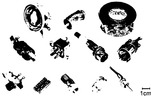
Figure 1.126. Components to avoid. We advise against using components like these, if you have a choice (see text if you need convincing!). Top row, left to right: low-value wirewound pot, type UHF connector, electrical tape ("just say no!"). Middle row: "cinch-type" connectors, microphone connector, hexagon connectors. Bottom row: slide switch, cheap IC socket (not "screw-machined"), type-F connector, open-element trimmer pot, phono connector.
